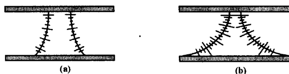
FIGURE 1. Schematic representation of possible director and optical axis configurations in hybrid aligned short pitch cholesteric system (a), (b).
